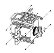
Start by attaching the plates to the camera. Make sure that the sides of the Mounting Plates (1) are aligned with each other.
